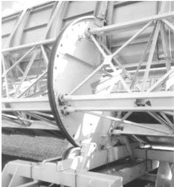
Figure 5: Close view of the wheel and the linear tracking mechanism.
